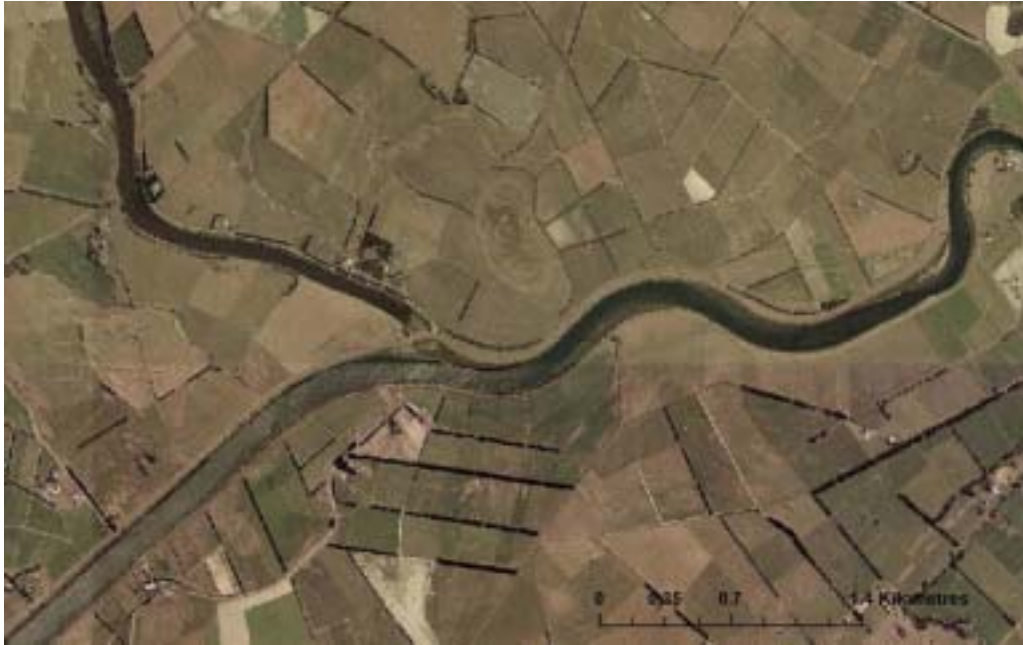
Figure 12: Aerial photo showing a section of the Lower Ruamahanga River reach 3. Note how the channel has been straightened and gravel beaches are largely absent.
