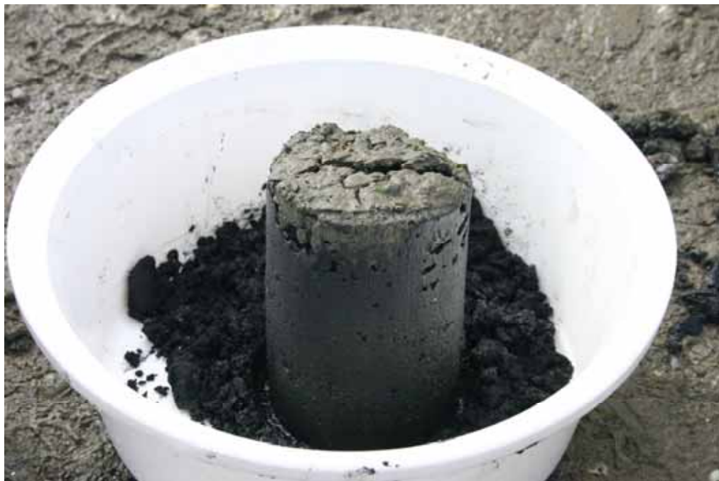
Figure 2.2: A sediment core sample taken from site POR-J, prior to removal of the top 20 mm
