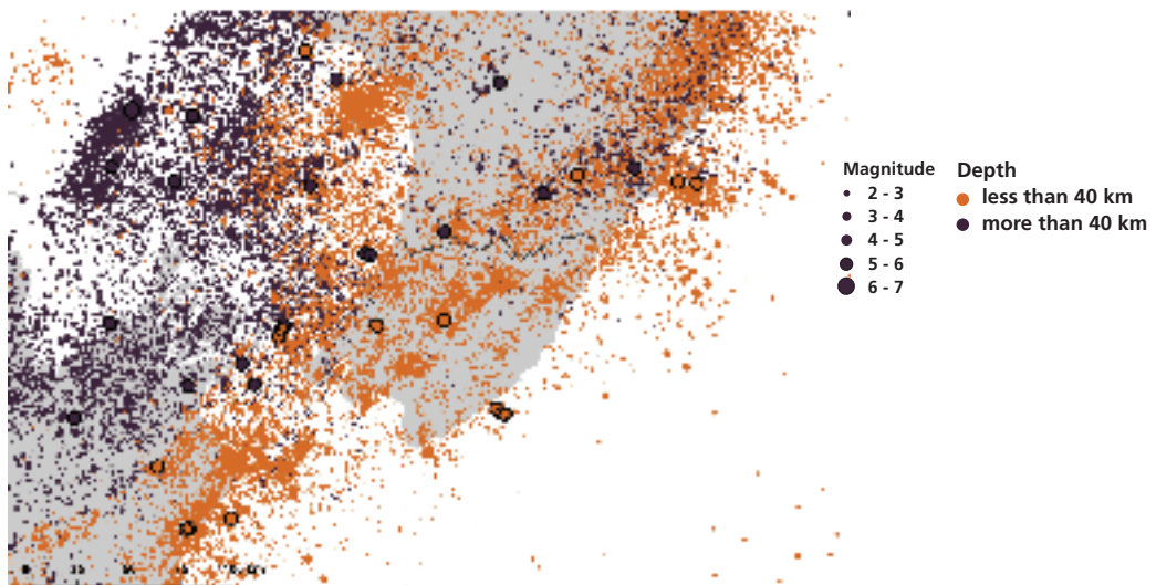
Figure 8.1: Earthquakes larger than magnitude 2 recorded in central New Zealand between 1995 and 2005. There is a general pattern of shallow earthquakes (less than 40 km deep) through Hawke's Bay, Wairarapa, Wellington and Marlborough, and deeper earthquakes – linked to the subducting, or sinking, Pacific Plate – from Taranaki to Nelson.
