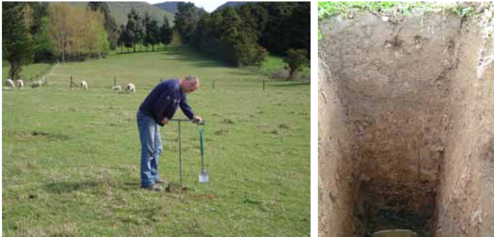
Figure 6.2: Scott Fraser (Landcare Research, left) using an auger to dig small cores to find an area of consistent soil type to sample at site PM006 and (right) soil profile at site PM013 consisting of silt loam topsoil, mottled silt loam to clay loam subsoil and an underlying compacted ironstone layer impeding drainage.
