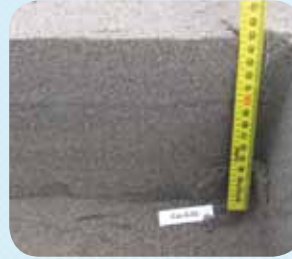
Measuring the depth of oxygenated sands
