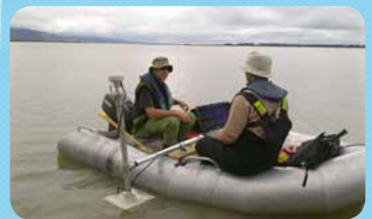
Staff using an echosounder (sonar) during a bathymetric survey of Lake Wairarapa
