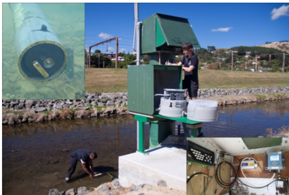
Figure 3.3: Porirua Stream at Town Centre flow and turbidity monitoring site. Top left inset: Turbidity sensor in the stream with lens and wiper showing. Bottom right inset: SC-200 control unit (top right) and data logger (top left) setup
