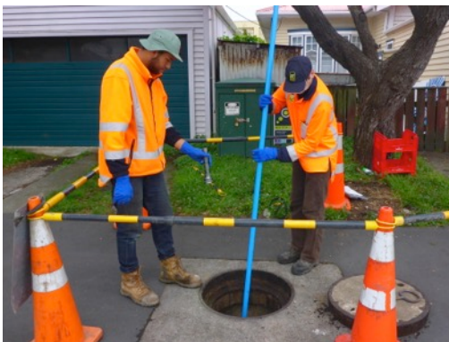
Using the extendable-handle kick net to collect a macroinvertebrate sample
