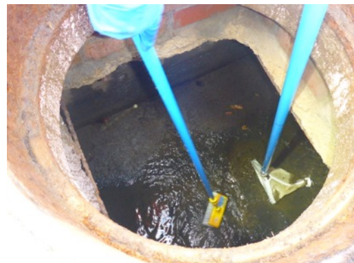
Using the extendable-handle kick net in conjunction with a brush to collect a macroinvertebrate sample
