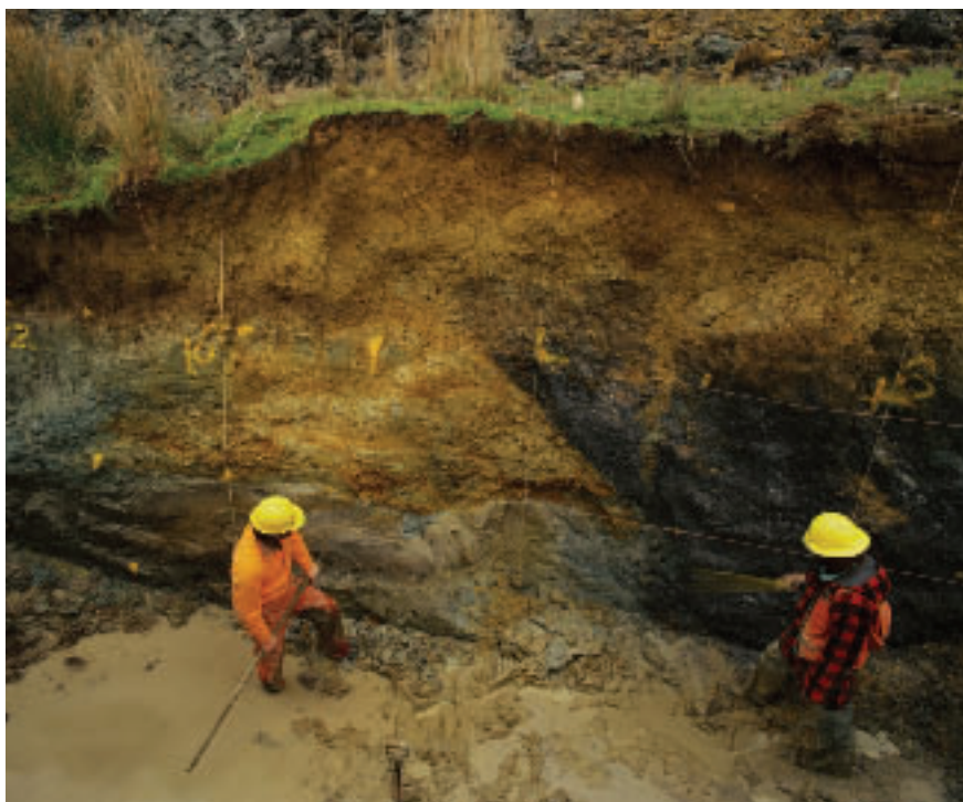
A trench across the Ohariu Fault in the Ohariu Valley - the land on the right hand side has been pushed over the land on the left hand side. Scientists date organic material in buried soil layers to determine when and how often the fault has moved. The Ohariu Fault last moved about 1100 years ago in an estimated magnitude 7.6 earthquake. Photo: GNS.
