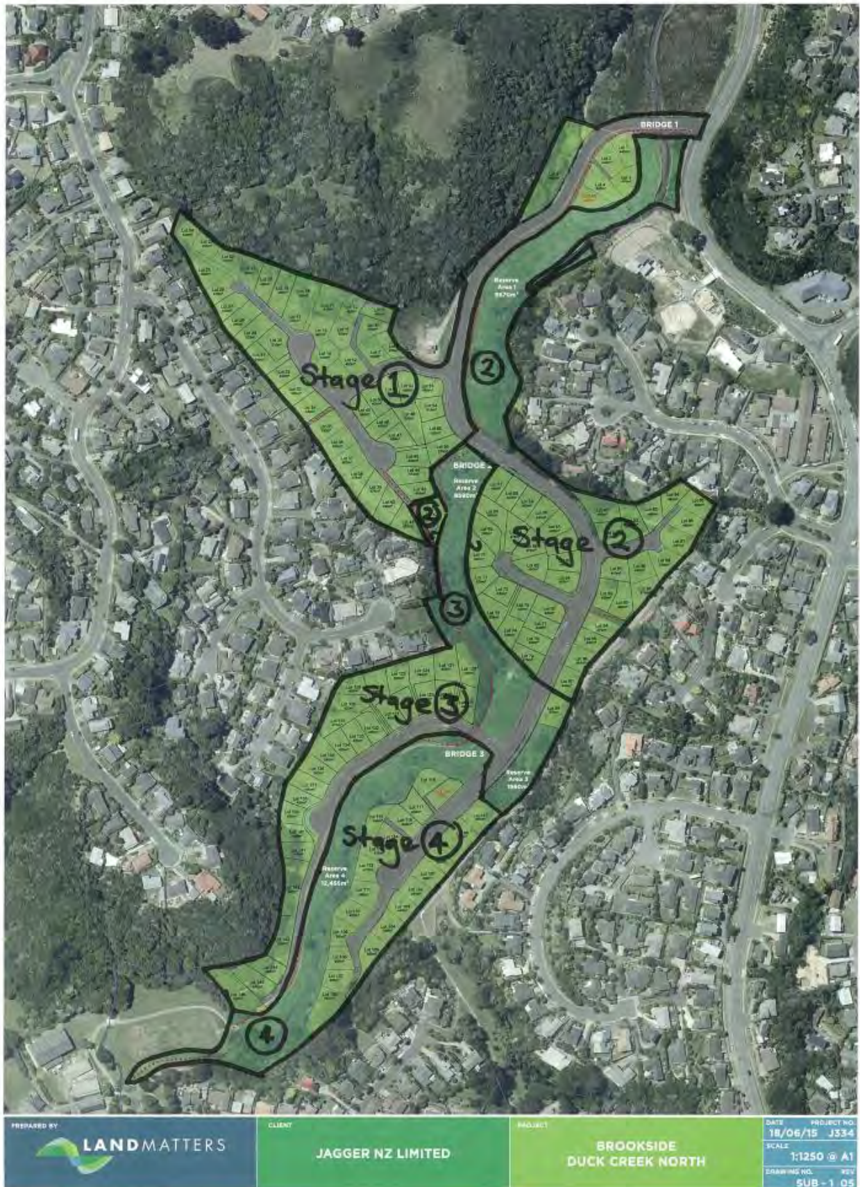
Figure 4 Duck Creek North Construction Staging
