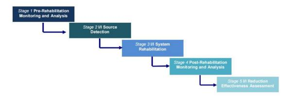
Figure 1: 5 stages of I&I reduction (NZ I&I manual 2015)
