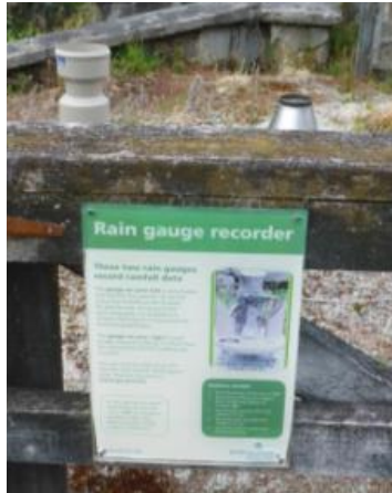
Telemetered rainfall gauge near Morton Dam, Wainuiomata
