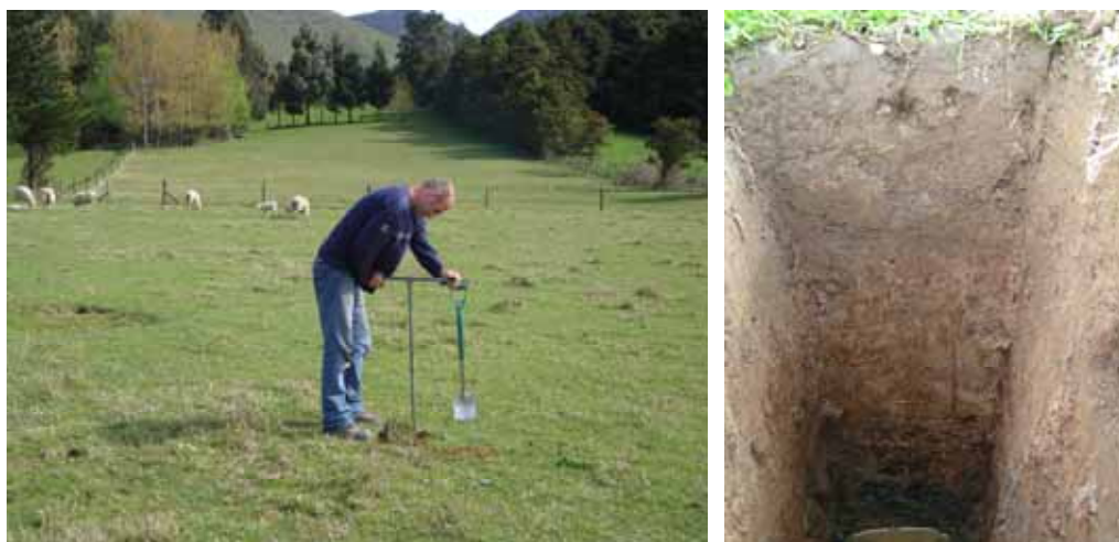
Figure 6.2: Scott Fraser (Landcare Research, left) using an auger to dig small cores to find an area of consistent soil type to sample at site PM006 and (right) soil profile at site PM013 consisting of silt loam topsoil, mottled silt loam to clay loam subsoil and an underlying compacted ironstone layer impeding drainage.
