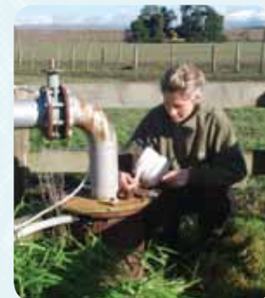
Checking the groundwater level
