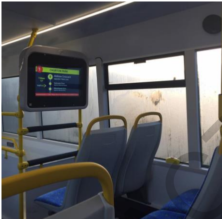
Fig 1: Condensation on windows in daytime
