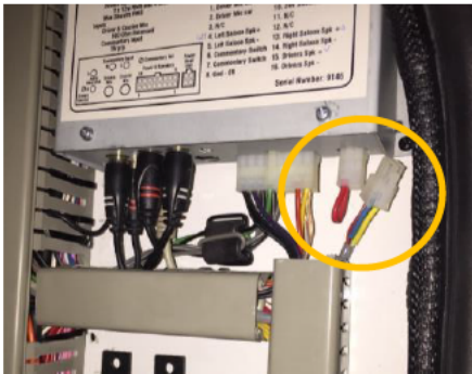
Fig 1: Solution to bypass stereo power control
