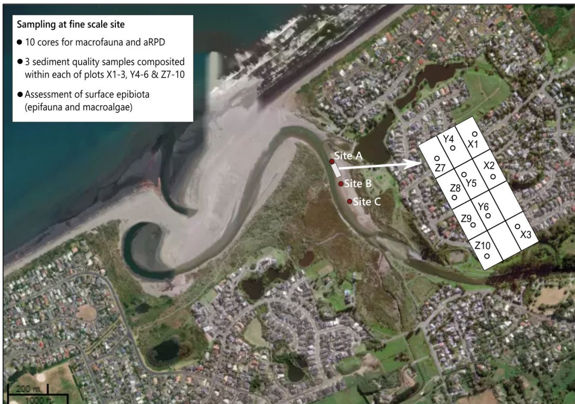
Fig. A1. Fine scale survey design at Waikanae Estuary monitoring sites. Sediment plates are installed at all sites (see Section B), but NEMP fine scale sampling is undertaken at Site A only (represented by rectangle).
