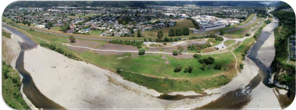
Figure 4. After development of Poets Park – plantings and wetted areas in foreground strip contaminants from urban, industrial areas and SH2 before reaching Te Awa Kairangi.
