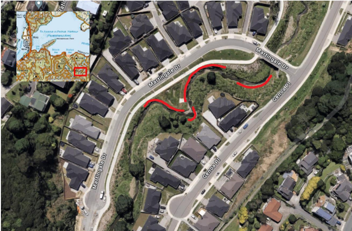
Figure 2: Wai-o-Hata/Duck Creek catchment, red lines show extent of rock lining. Source: Natasha Petrove, DOC Technical Advisor Freshwater, based in Wellington.
