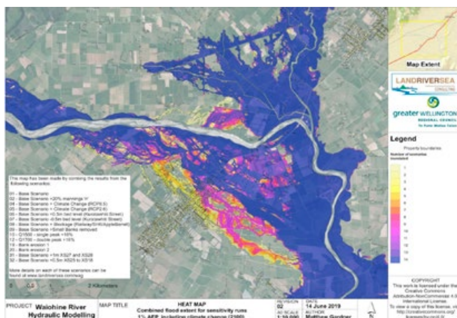
Figure 36: Significant flood sensitivity scenarios laid one on top of another to see maximum extent – landriversea Consulting.
