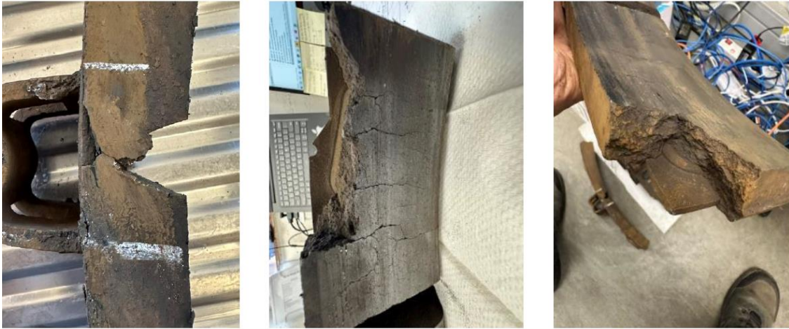
Brake blocks from myriad carriages; the failure mode is new
