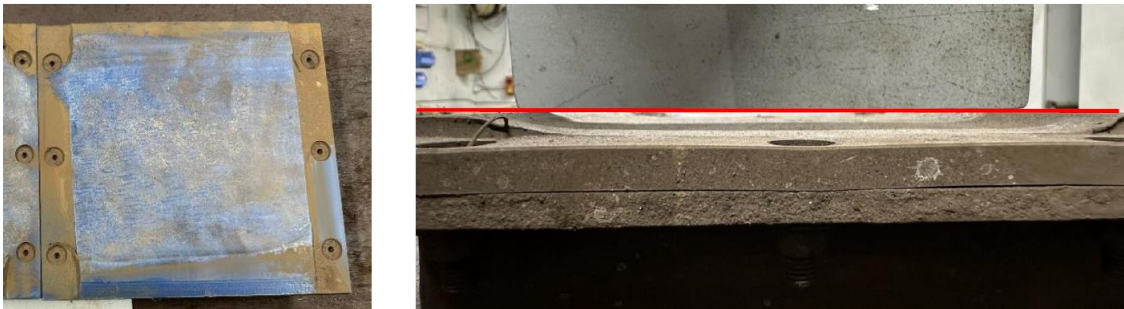
Worn wear liners with a very rough finish. Normally they are smooth and evenly worn
