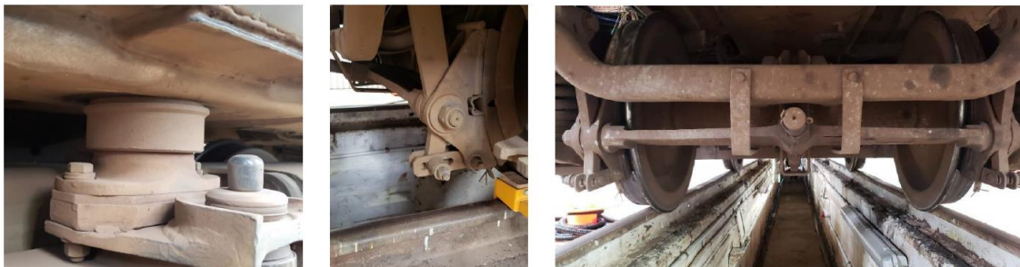
The bogies on SW3394 show much less evidence of fretting
