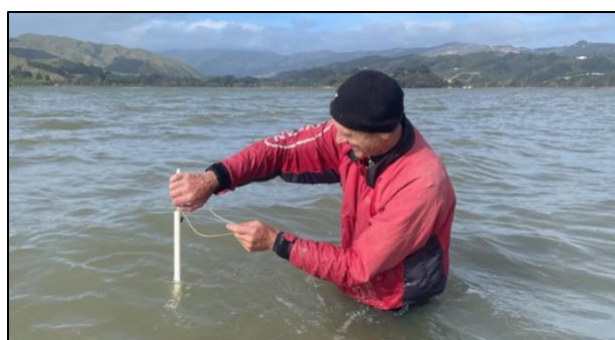
Frame used to measure subtidal plates (top) and measuring a subtidal plate at the water surface (bottom).
