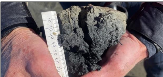
25mm of oxygenated sand above organically enriched sediment Onep B (O3), Onepoto Inlet.
