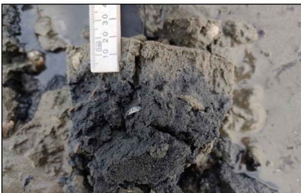
The depth to a visually obvious colour change is used to assess oxygenation in sediment.
