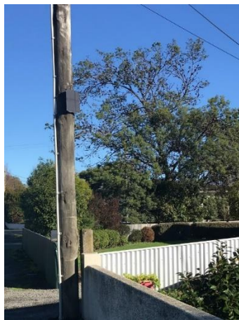
Figure 7.6: Solar powered NIWA ODIN PM 2.5 monitor containing a PMS3003 dust sensor mounted on street pole in Masterton, winter 2020
