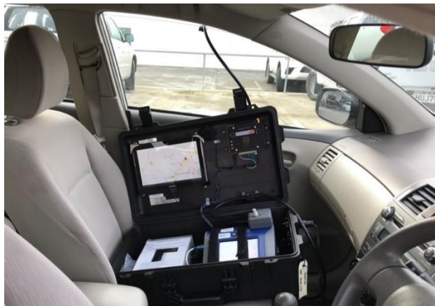
Figure 7.4: SmokeTrak (Kenelec Scientific) measuring system using a TSI DustTrak Aerosol Monitor (model 8533) with an in-line PM 2.5 filter housed in a travel case together with a GPS sensor, a modem and a tablet for displaying measured PM 2.5 concentrations
